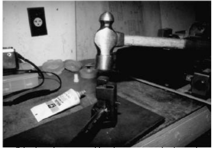
Crimping a lug onto a cable using a proper crimping tool.
