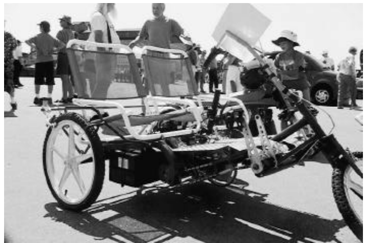
Don Crabtree's other creation, a brand new lightweight power-assisted tandem recumbent. (Gordon Wong)
