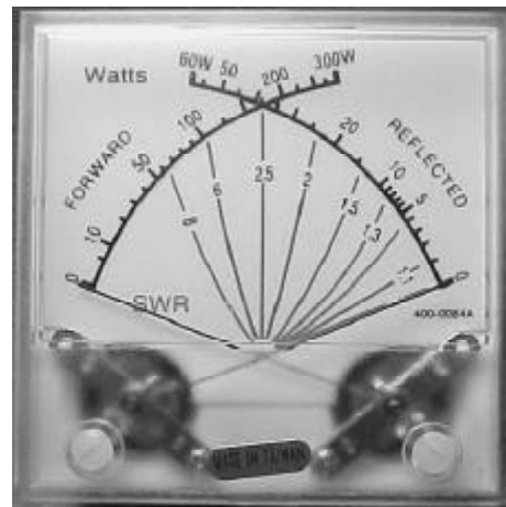
This is the cross-needle meter movement as received from MFJ.
